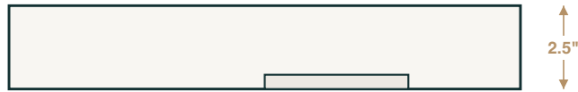
RE section shown (2.5" — carries the 24 V connection box); AC section 1.5" (integral driver).
